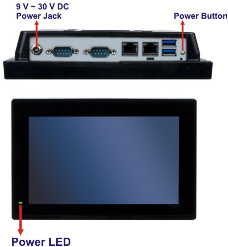
Figure 3-25: Powering On the System
