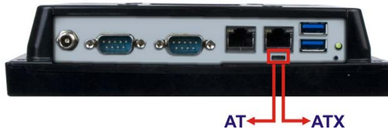
Figure 3-5: AT/ATX Switch Location
