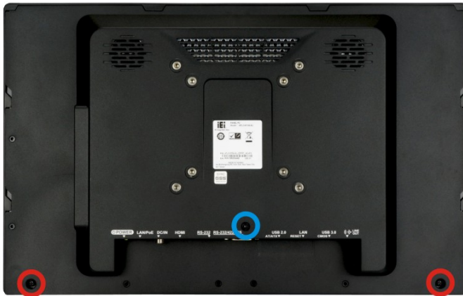
Figure 3-3: AFL3-W15A-AL Back Cover Retention Screws
