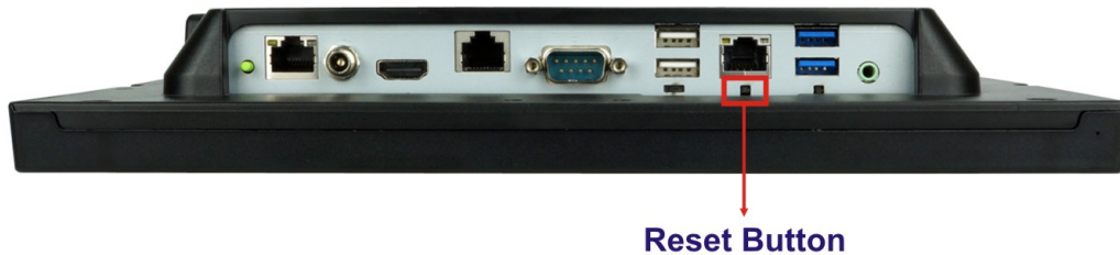
Figure 3-42: Reset Button Location
