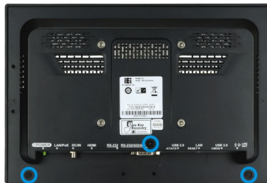
Figure 3-1: AFL3-W10A-AL Back Cover Retention Screws
