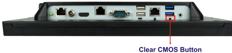
Figure 3-41: Clear CMOS Button Location
