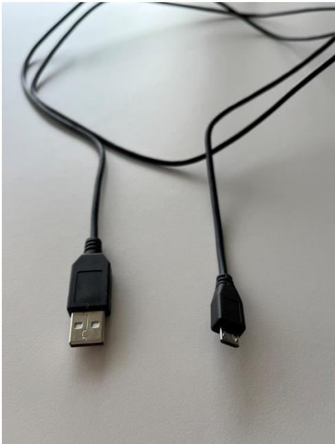
Connect the Tableaux to your computer with a USB cable (USB type A to micro USB type B) as the one shown in picture
