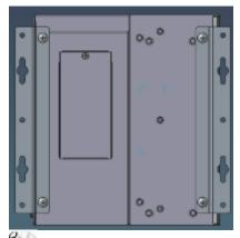
Note: When using this wall mounting (1) in IPC with internal fan module, considering fan air flow, a space must be left between system and wall.
