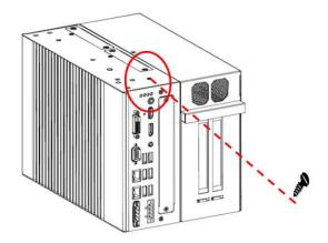
Step 5 Insert the module to slot and push it down firmly.
