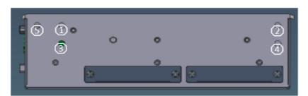
Step 7 Close the heatsink cover to the chassis and fasten all screws. The installation is complete.
