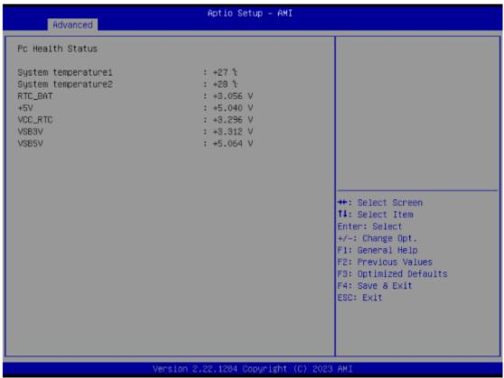
This screen displays the temperature of system and CPU, cooling fans speed in RPM and system voltages (VCC\_CPU, DDR, +12V, +5V and +3.3V).
