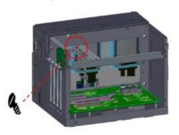
Step 10 Close the cover back to the chassis and tighten the screw. The installation is complete.
