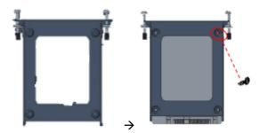
Step 5 Insert HDD tray to main box, then screw 2 screws for each HDD tray. Installation is complete.
