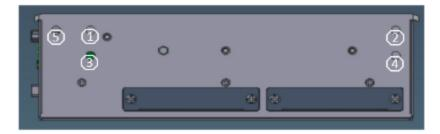
Step 8 Close the heatsink cover to the chassis and fasten all screws. The installation is complete.
