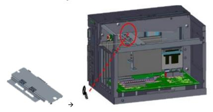
Step 7 IPC962A and IPC964A offer 3 types of extension holder brackets. Please take the brackets and screws from the accessory box and assemble the extension holder bracket. The procedure is illustrated below.
