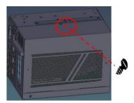
Step 4 Loosen the screw to remove the bracket.
