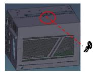
Step 4 Locate the PCI or PCIe slots and remove the slot bracket from the slot in which you want to add the card.
