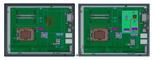
Step 6 Remove the antenna plug(s), and then screw the antenna(s) on the system.
