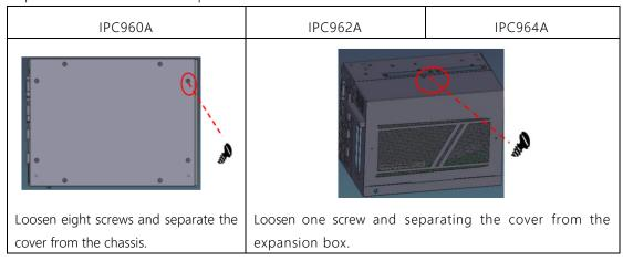
Step 4 Remove the expansion box as shown below.
